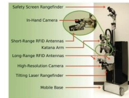
Home robotics combine information from multiple sensors on the robot and in the environment.
